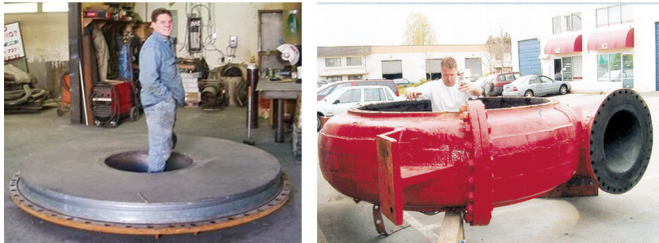
CTI Wear Lining on a 28 inch Dredge Pump and Suction Liner.
