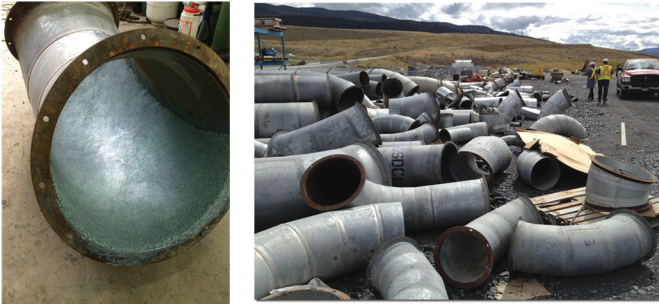
Overhauled Dust Collection Pipe components - currently running over 3 years with no noticeable wear that offers over 20 times the normal unprotected life expectancy.
