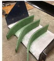
Overhauled Dirty Paddle Fan that was subjected to dust particulates. CTI Lining has proven effective more than 8 times its life expectancy.
